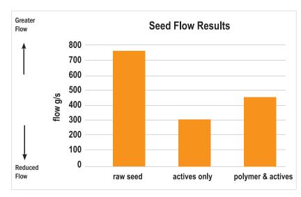
The above graph shows the difference seed flow before and after a treatment, and with the same treatment when using a polymer coating.
